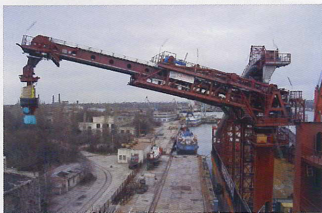
Shiploader installed on the Bulk Kremi. Photo courtesy of Coeclerici Logistics.
