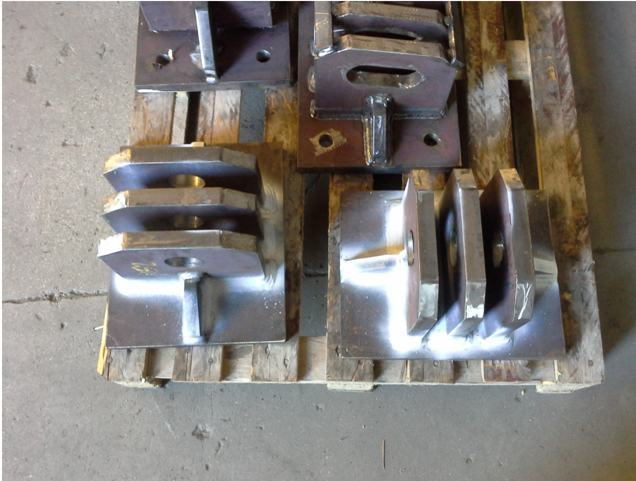
Welding test by Liquid Penetrant Test (LPT)
