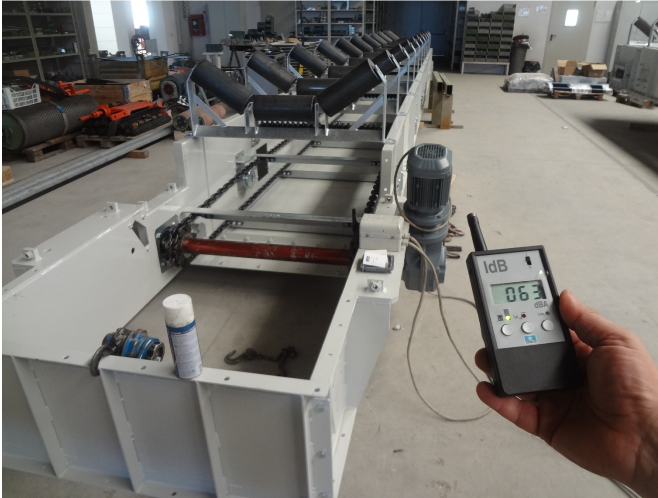
Noise measurement of spill chain in SAMMI Factory
